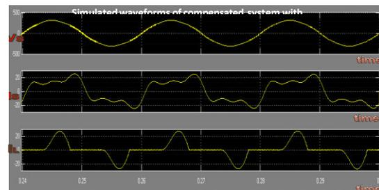
To further reduce the value of the THD, the active filter is placed in the circuit with the dc capacitor voltage of 85V. Fig. 10 shows the simulation results for this case. The THD of the power source current ( $i_s$ ) reduced from 41% in off-line active filter mode to about 2.75%.
