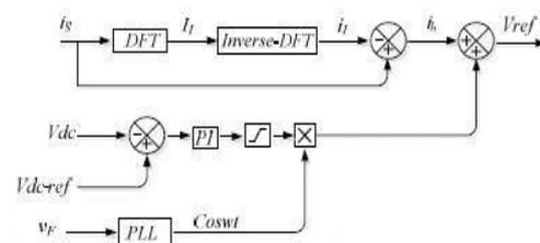
Fig. 2. Control circuit of hybrid series active filter.
