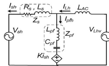
Fig. 7. Harmonic equivalent circuit of single phase system.
