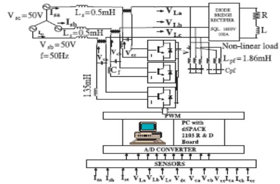
Fig 1. Schematic diagram of the control and power circuit of the HSAPF.
