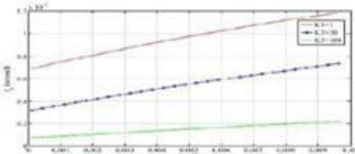
Fig. 5. Relationship between system critical time and system impedance.
