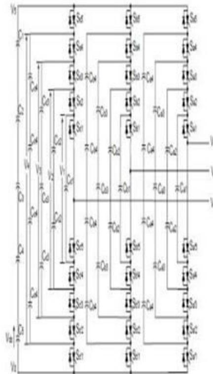
Fig 2. Three-phase six-level structure of a flying capacitor inverter.
