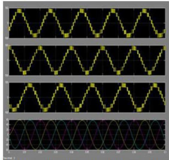
Fig10 output voltages and currents of Three-phase five-level diode clamped inverter.
