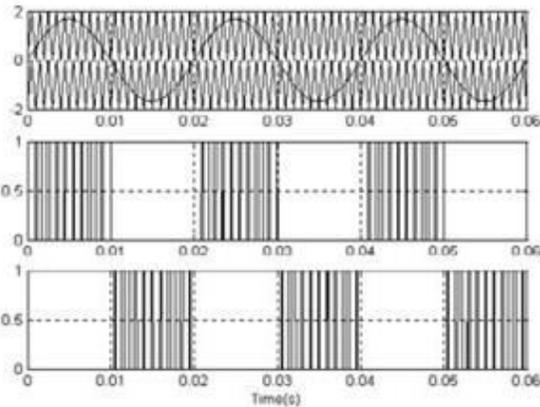
Fig.8 pulse generation for 3-level inverter (for switches Sa1&Sa2).
