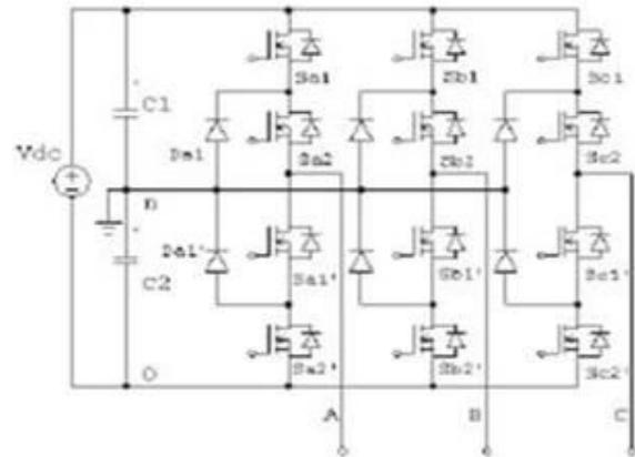
**Fig.5. Three phase three level diode clamped inverter**
