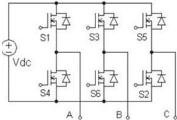
**Fig.4 Three-phase two-level inverter.**
