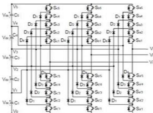
Fig.1. Three-phase six-level structure of a diode-clamped inverter
