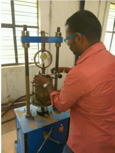
Figure-3 C.B.R Set up
