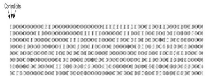
Fig 6. Parity check matrix for a minimum weight SEC code that protects 128 data bits and 3 control bits.
