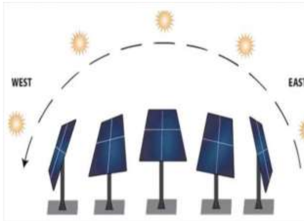
Fig.2. Sun's position for Dual-Axis tracking
