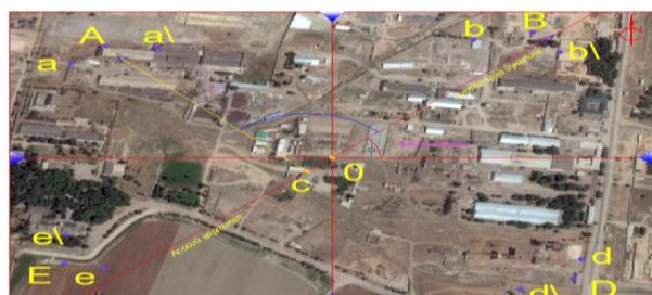
Fig1. The location of the points in the aerial photograph is distorted by the deflection angle
