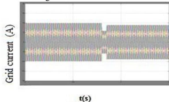
Fig.11. Three-phase grid current waveforms with modulation compensation.
