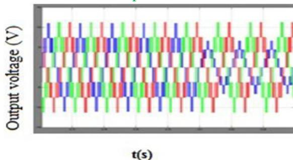
Fig.12. Three-phase inverter output voltage waveforms with modulation compensation.
