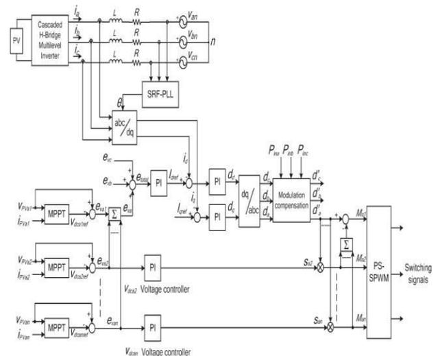
Fig. 3. Control scheme for three-phase modular cascaded H-bridge multilevel PV inverter
