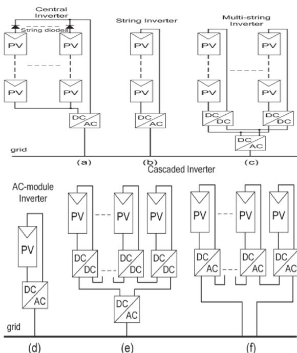
Fig.1. Configurations of PV systems. (a) Central inverter. (b) String inverter. (c) Multistring inverter. (d) AC- module inverter. (e) Cascaded dc/dc converter. (f) Cascaded dc/ac inverter.
