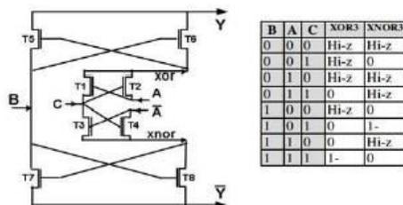
Fig 1: BC1 circuit and input and output values
