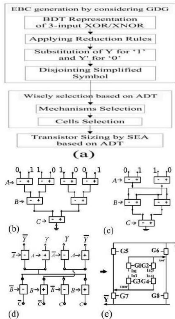
Fig. 6: (a) SCDM process for designing efficient three-input XOR/XNORs. (b) BDT representation of three-input XOR/XNOR function. (c) Applying reduction rules. (d) Substitution and disjointing. (e) EBC.
