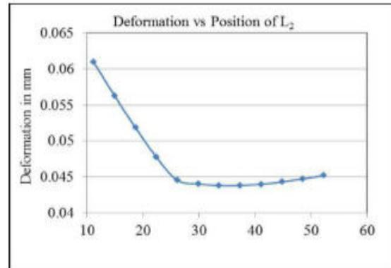
Figure 1.5 (b) Position of Locator L<sub>2</sub> vs workpiece deformation
