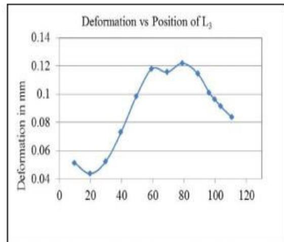
Figure 1.5 (c) Position of Locator L<sub>3</sub> vs workpiece deformation
