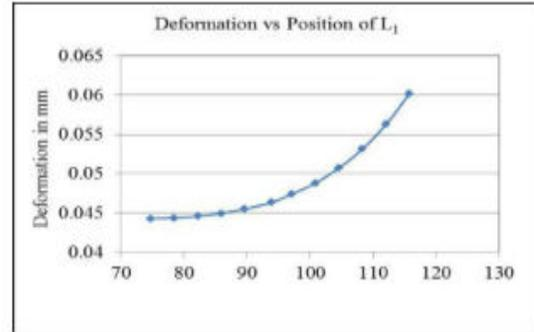
Figure 1.5 (a) Position of Locator L<sub>1</sub> vs workpiece deformation
