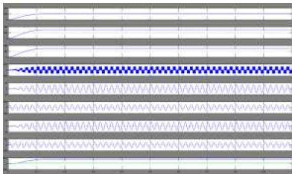
Fig2. Pv voltage current and power , inverter voltage, grid voltage, grid current, load voltage, load current, dc link voltage and current
