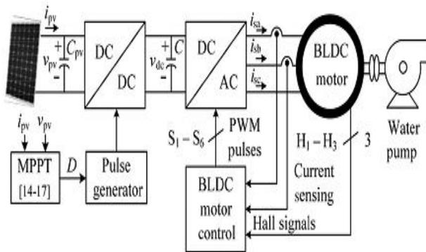
Fig.1. Conventional SPV-fed BLDC motor-driven water pumping system
