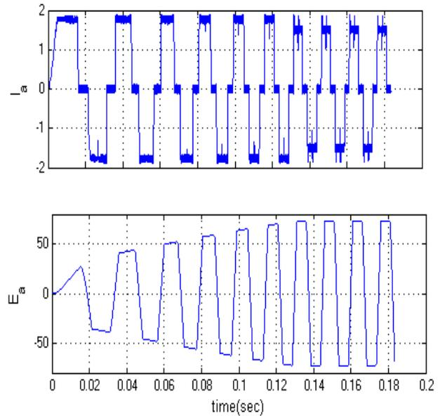
Fig.11 Stator current and emf.
