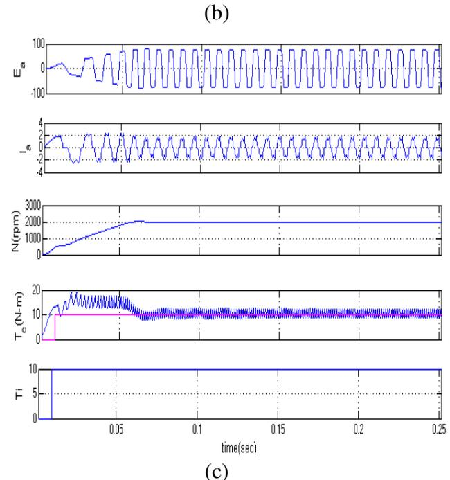
Fig.5 Starting and steady-state performances of the proposed SPV array based zeta converter-fed BLDC motor drive for water pump. (a) SPV array variables. (b) Zeta converter variables. (c) BLDC motor-pump variables.
