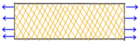
Direction of Loading in In-Plane Shear
