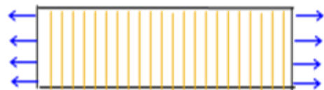
Direction of Loading in Transverse Tensile
