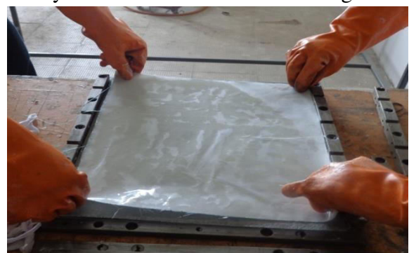
Placing first the ply
