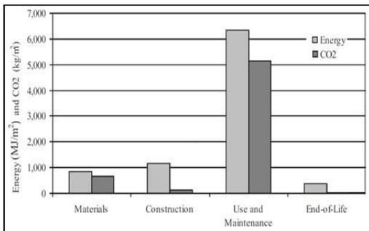
Fig. 4. Energy and CO<sub>2</sub> by life cycle stages [20]
