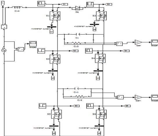
**Fig 4. Matlab/Simulink Diagram of Existing Multi Output PFC Rectifier System**
