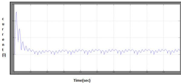
**Fig 11. DC motor current**
