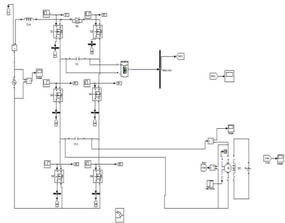
**Fig 9. MATLAB/SIMULINK diagram of proposed multilevel rectifier with battery and dc motor**
