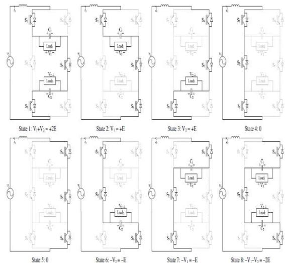
**Fig.2. Operating sequences and conducting paths of proposed HPUC 5-level buck rectifier**
