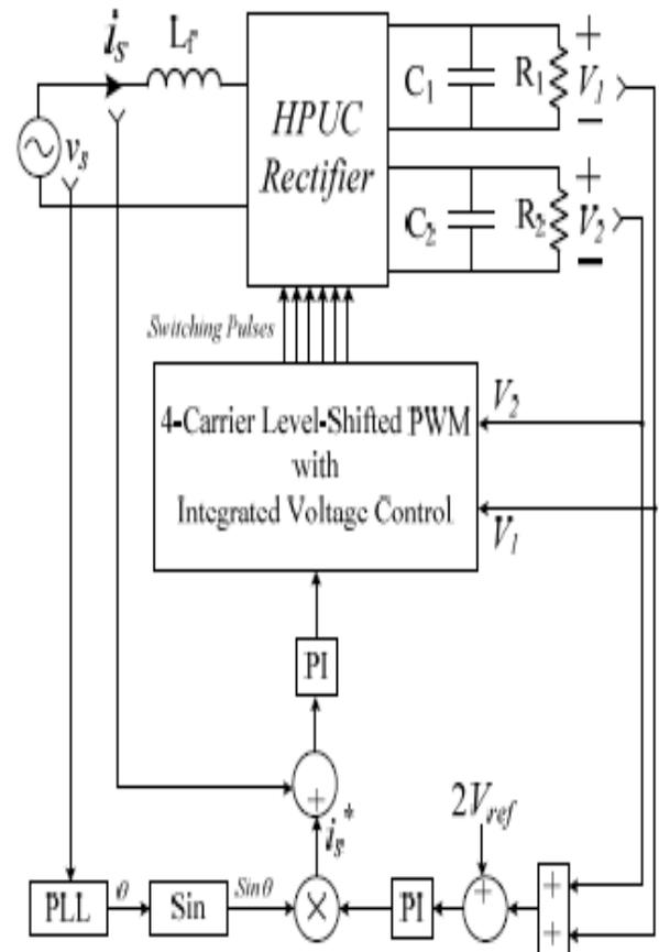
**Fig 3. Block diagram of the HPUC rectifier and Implemented controller**
