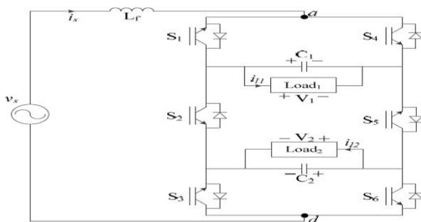
**Fig1. Proposed HPUC five-level buck PFC rectifier**
