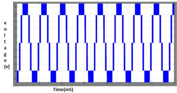
**Fig 14. Five level rectifier voltage**
