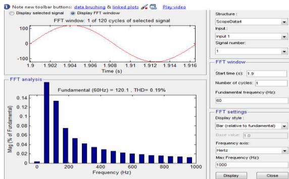
**Fig13. THD% of voltage of rectifier**
