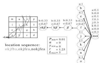
Fig. 2. An example of an object's moving trajectory, the obtained location sequence, and the generated PST  $T$ .
