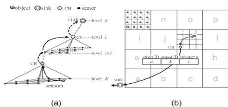
Fig. 1. (a) The hierarchical- and cluster-based network structure and the data flow of an update-based tracking network. (b) A flat view of a two-layer network structure with 16 clusters.
