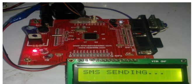
Figure 10. Implemented circuit (Showing sending SMS)
