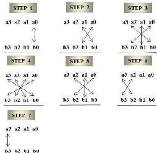
fig.4: multiplication of two 4 bit numbers using urdhvatiryakbhyam
