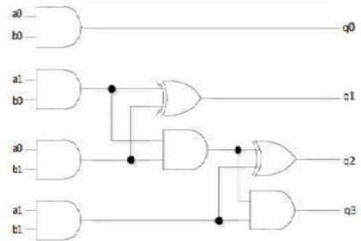
Fig. 6: 2\*2 Vedic multiplier using conventional gates.
