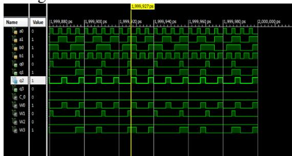
Fig.10: Simulation results for reversible 2\*2 Vedic multiplier.
