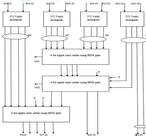
Fig.9: Block diagram of Reversible 4\*4 Vedic multiplier.
