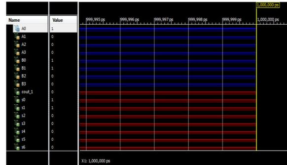
Fig.11: Simulation results for reversible 4\*4 Vedic multiplier.
