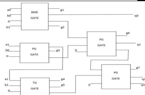
Fig. 7: proposed 2\*2 Vedic multiplier using Reversible logic gates.
