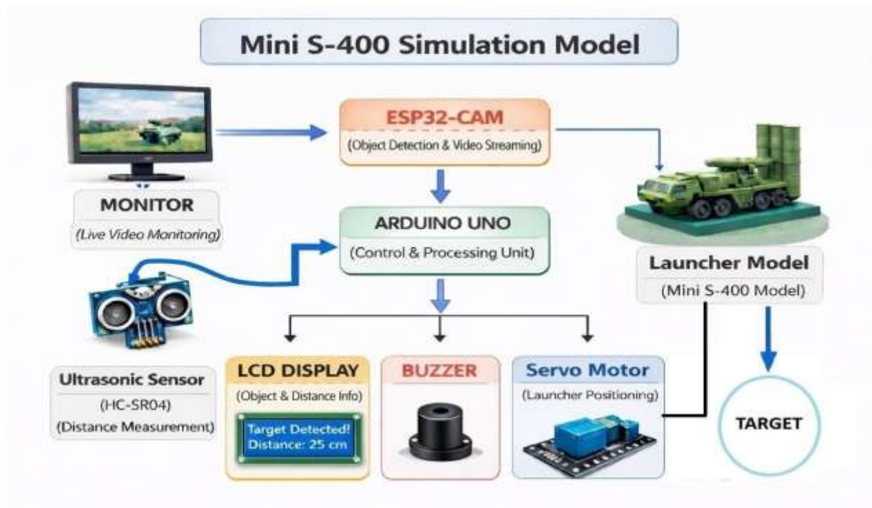
Fig. 1 illustrates the overall architecture of the proposed Mini S-400 automatic detection and tracking system.
