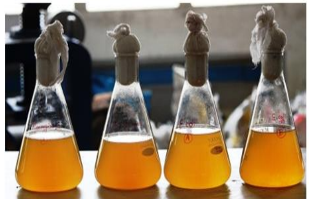
Figure 2.4: 800 ml P. Aeruginosa , B. Subtilis and E. coli culture media for concreting
