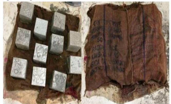
Figure 2.7: Jute bag curing of concrete cubes
