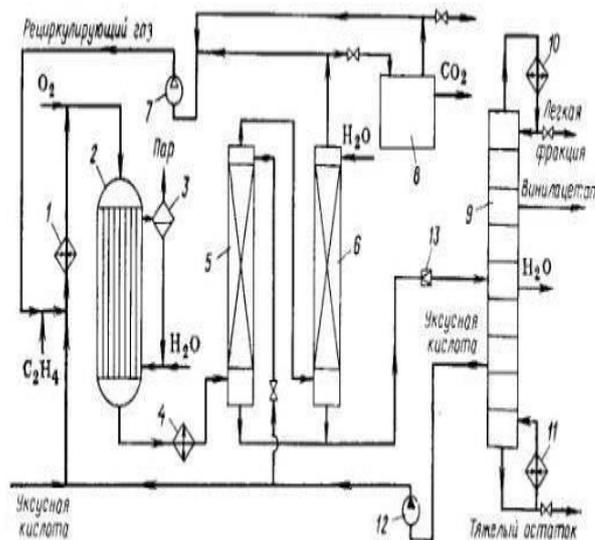
Figure 1. Technological scheme for the production of vinyl acetate from ethylene
