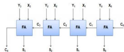
Fig 2: Ripple Carry Adder
