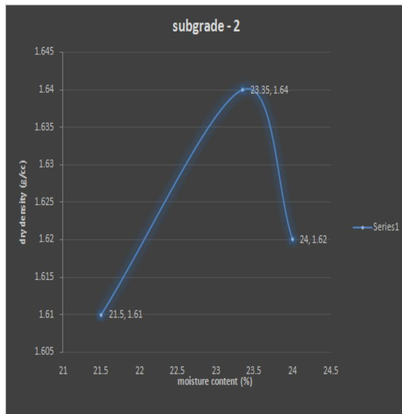
**Fig 4.2 S the compaction test results on sub grade soil (sandy soil)**
