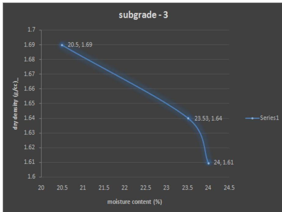
**Fig: 4.3 shows the compaction test results on sub grade gravel**
