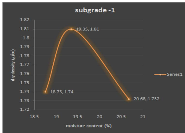
**Fig: 4.1 Shows the compaction test results on sub grade soil (clay)**
