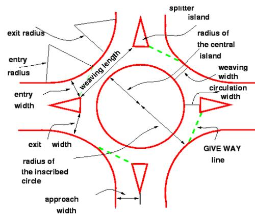
Fig 1: Design elements of a rotary
