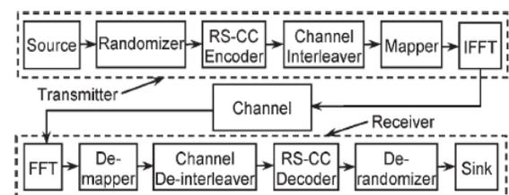
**Fig. 1. Block diagram of the WiMAX transceiver.**
