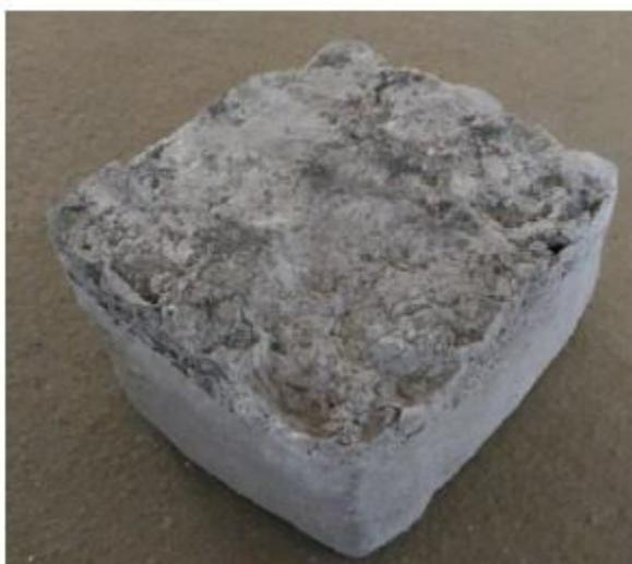
Fig.2: Aluminium 6351 Precursor obtained after solidification
