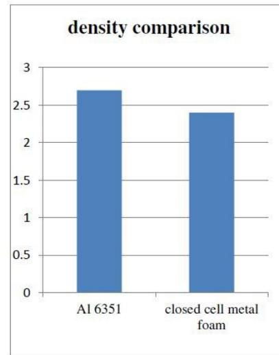
Fig 5: Variation of density in Al 6351 and developed foam
