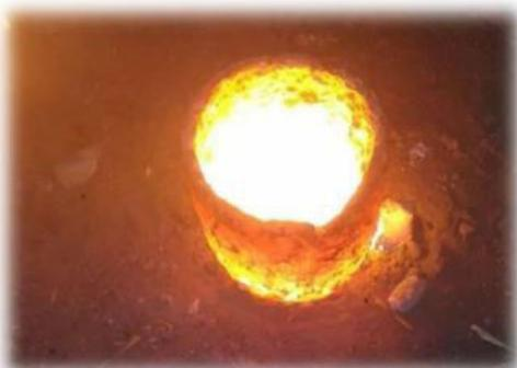
Fig. 1: Molten Aluminium 6351 in crucible
