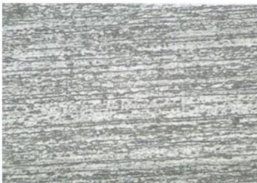
Fig.4 (a): Optical microscope image of parent metal
