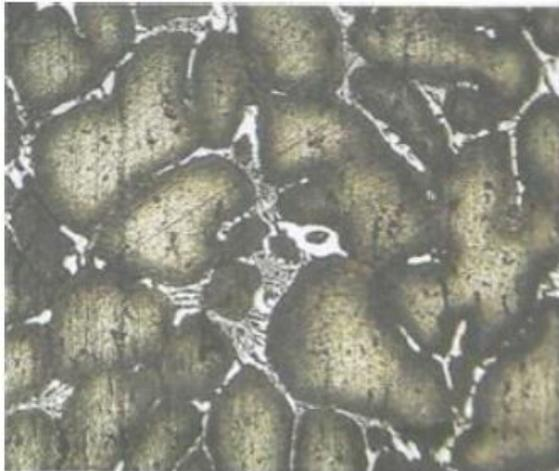
Fig.4 (b): Optical microscope image of closed cell Al 6351 foam
