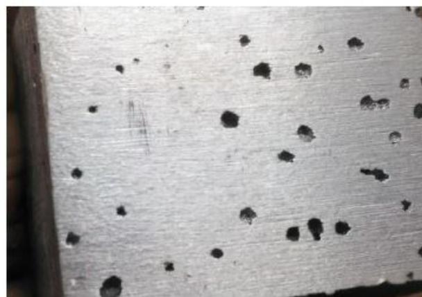
Fig.3: Aluminium 6351 foam obtained after annealing
