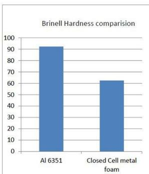
Fig.7: variation of Brinell hardness in Al 6351 parent metal and developed foam
