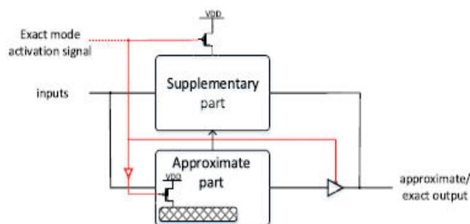
Fig. 1. Square graph of the proposed estimated 4:2 blowers. The achured enclose the estimated part shows the segments, which are not shared among this and strengthening parts.
