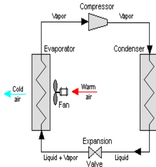
**Fig. 4.1 Schematic diagram of the experimental setup**
