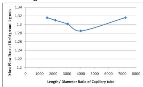
Graph.2 Effect of L/D of capillary tube on Mass flow rate of refrigerant
