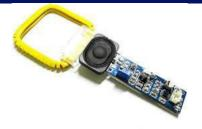
This is a metal detector with a speaker and TTL output. A metal detector is an electronic instrument
