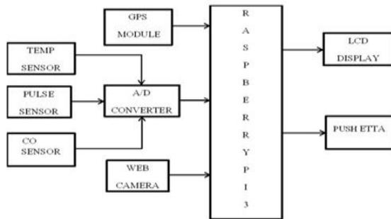
Fig 2.1 Block diagram of system
