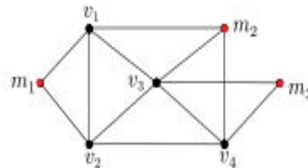
Fig.3.1. Sample network with three monitors: m1, m2, and m3.
