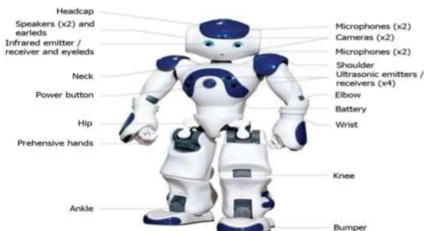
Fig 1: Humanoid Robot Structure
