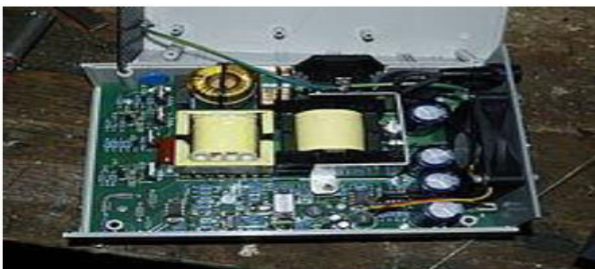
Fig2. Inside of a SWEA 250W Transformer-based grid-tie inverter.
