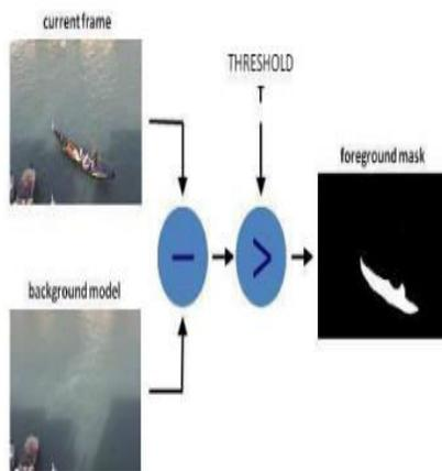
Fig. 3 Example of Background subtraction method
