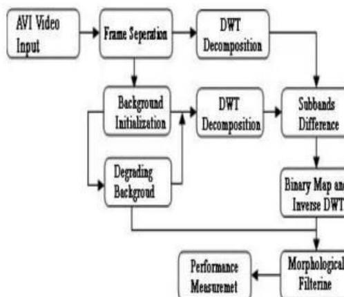
Fig.5 Block diagram for proposed method
