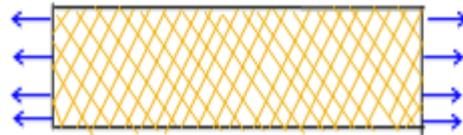
Direction of Loading in In-Plane Shear
