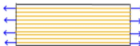
Direction of Loading in UD-Tensile
