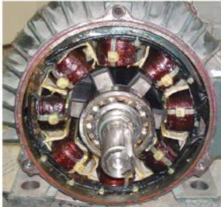
Fig.3 The tested 8/6 SRM inside view
