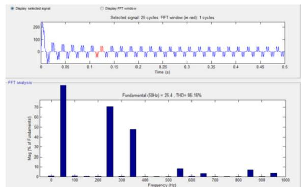
Fig.13 Harmonic analysis of closed loop SRM is 86.16%
