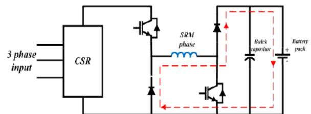
Fig.6 Battery Charging in Regenerative Mode of SRM
