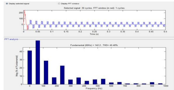
Fig.18 Harmonic analysis of closed loop SRM is 40.48%
