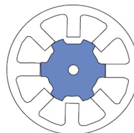
Fig.1 shows the 4-phase,8 rotor poles/6 stator poles
