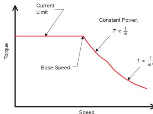
Fig.3 SRM Torque-Speed Characteristics
