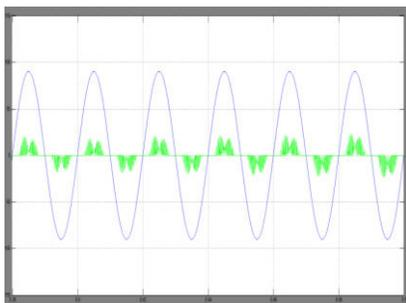
Fig.15 Simulated input wave form of Voltage and current for closed loop controlled SRM Drive
