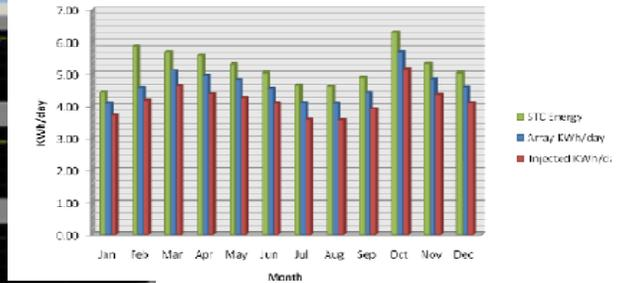
Fig 8: Monthly energy generation from 1kWp PV system throughout the year
