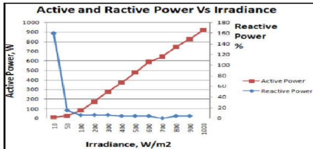
Fig 10a) Active and reactive power variation at inverter output
