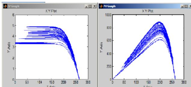
Fig 5: IV and PV curve of array with RL load and time varying input
