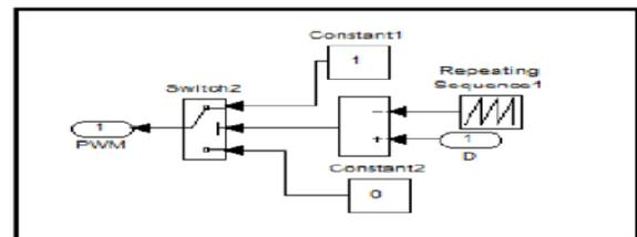
Fig 3: Model for MPPT: Simulink model for PWM wave generation
