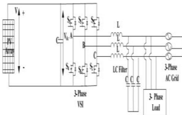
Fig 1: General Block Diagram of Grid Connected SPV system
