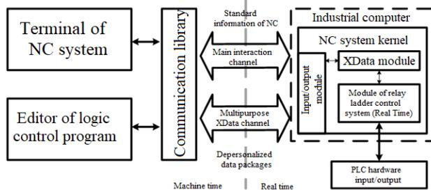
Fig. 2. The architecture of NC system with embedded software controller
