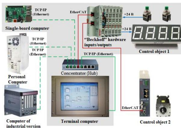
Fig. 1. Network model of the experimental bench for testing the performance of logical control systems
