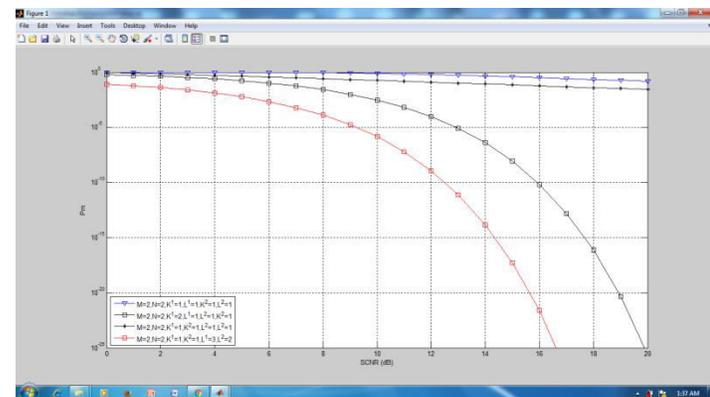
FIG: Miss detection probability versus SCNR for 2x2 MIMO-OTH radar with different number of forward paths and backward paths
