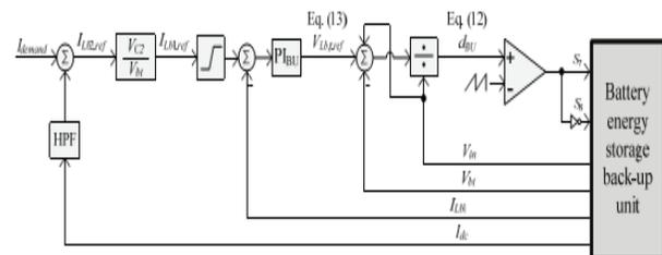
Fig 7 (b). The control block diagram of the three phase three line with battery energy storage back up unit
