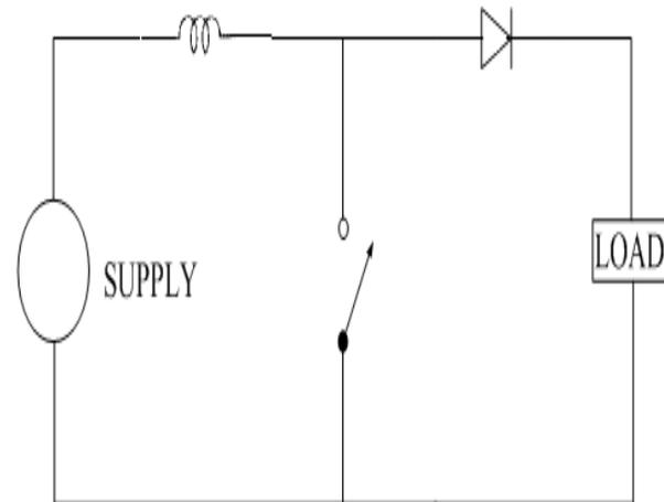
Fig.3 basic boost converter circuit diagram
