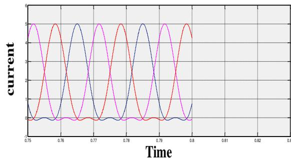
Fig.12 Simulation result for Inductor currents
