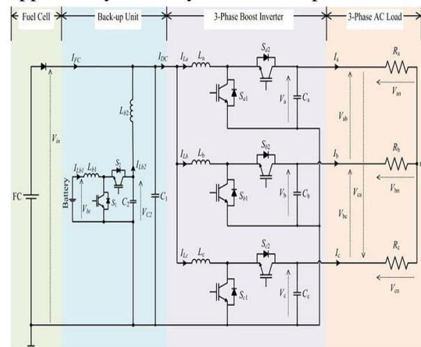
Fig.6 three-phase FC stand-alone power supply using only a single energy conversion stage including a back-up unit with battery storage
