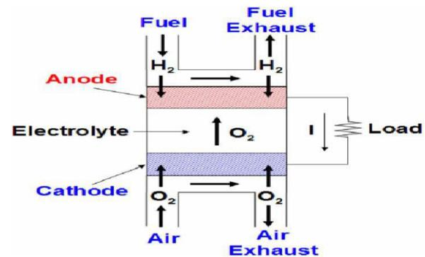
Fig.2 Fuel cell overall operational diagram
