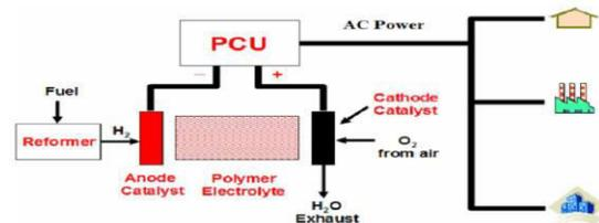
Fig.1 Fuel cell block diagram
