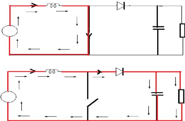
Fig.4 switching operation circuit of boost converter
