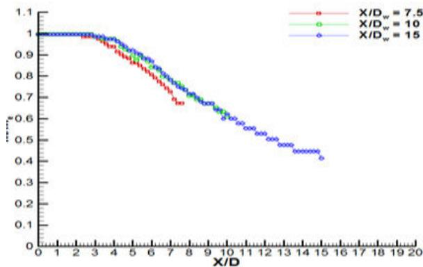
it is seen that the Mach number 0.4 free jet core length is little longer than other impinging jets. Here impinging jets  $X/D_w = 7.5, 10$  are propagating almost similar in the decay at  $X/D = 3$  onwards. Free jet and impingement jets behave in the similar fashion in the far field.
