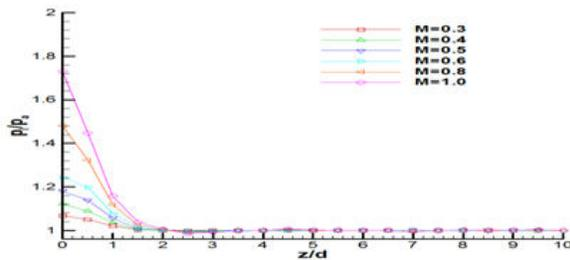
Wall pressure distribution at impingement location  $X/D = 5$  for various jet Mach numbers.
