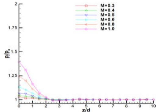
Wall pressure distribution at impingement location  $X/D = 10$  for various jet Mach numbers.
