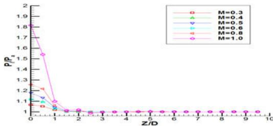
Wall pressure distribution at impingement location  $X/D = 1$  for various jet Mach numbers
