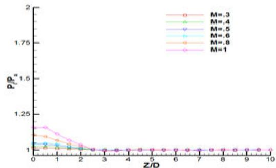
Wall pressure distribution at impingement location  $X/D = 15$  for various jet Mach numbers.
