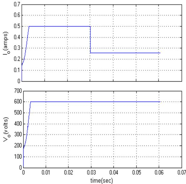
Fig.11 Voltage and Current wave forms with sudden decreasing load
