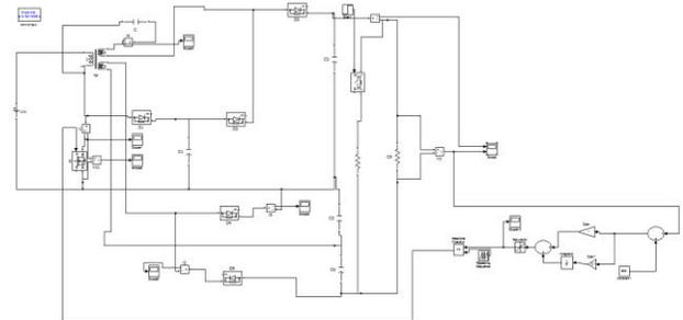
Fig.9 simulink model of step-up dc-dc converter with closed loop control
