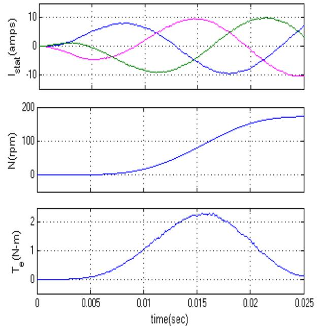
Fig.14 Stator current, Speed, Torque characteristics of the induction motor
