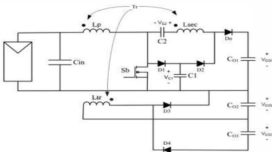
Fig.2. Proposed High Step-Up Converter.
