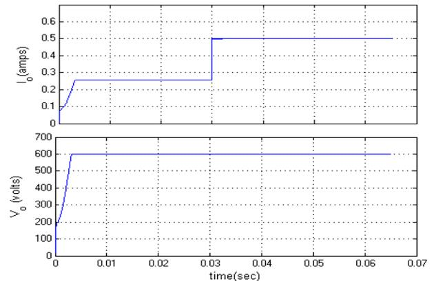
Fig.10 Voltage and Current wave forms with sudden increasing load
