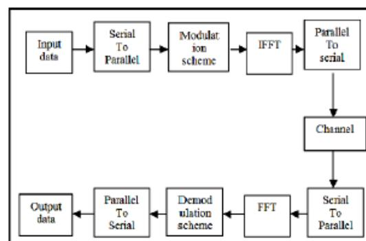
Fig 1: Block Diagram of FFT Based OFDM System
