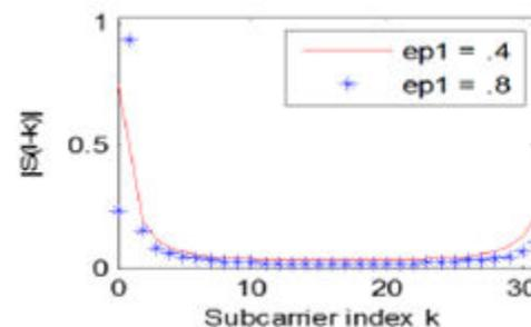
The figure 2 shows that for a larger  $\varepsilon$ , the weight of the desired signal component,  $S(0)$ , decreases, while the weights of the ICI components increases. We can notice that the adjacent carrier has the maximum
