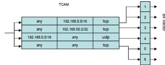
Figure 1: TCAM for Compressed Header Rules
