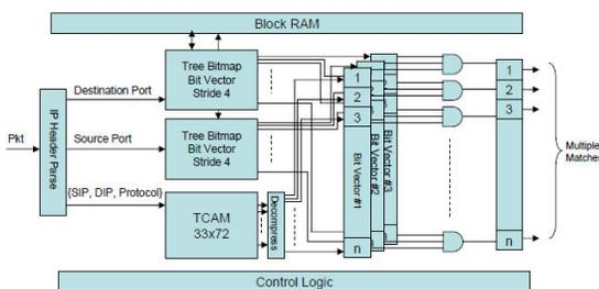
Figure 3: BV-TCAM Circuit Block Diagram in XCV2000E
