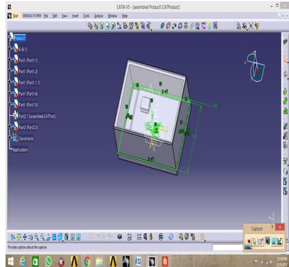
It is a hollow enclosed rectangular box of 150x110 mm<sup>2</sup> having a wall thickness of 5mm.
