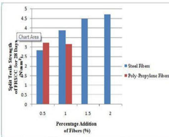
Fig.4.2: Split Tensile strength of FRSCC for 28 Days
