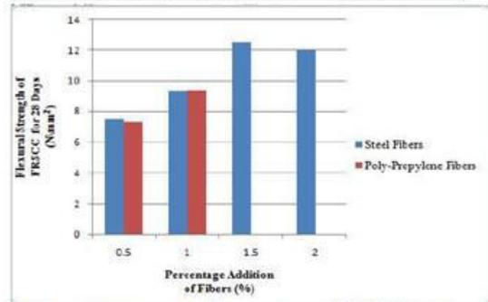
Fig.4.3: Flexural Strength of FRSCC for 28 Days
