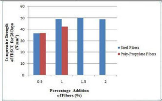
Fig.4.1: Compressive Strength of FRSCC for 28 Days
